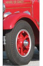
Wheels, wheels wheels: We are working on wheels and going many places! We started with two projects and ended with four. The 1899 American steamer (center and top right) wheels have been completely re -done since 2011. Three layers of designs were recorded and removed. Paint color was matched to the original and 5-6 coats of enamel were applied by brush. Then in April of 2013 two sets of 'decals' made by Ken Soderbeck were attached. Days later, master
